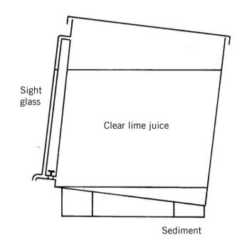
Figure 2: Lime juice clarification using the tilted tank method - Illustration: Practical Action
